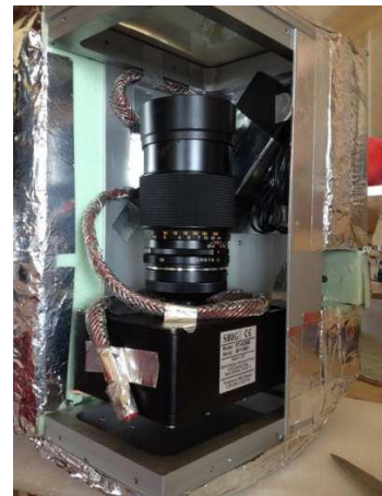
Left: tests on the pointing system observing SuperDARN container (upper-right image on the screen) – Right: CCD camera with heating cables and foam insulation.
