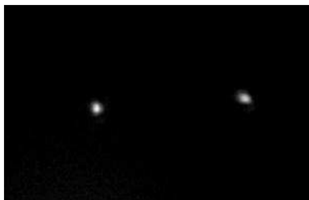
Fig. 1: Left, the DIMM system. Note the 2 hole mask at the telescope top. The box at telescope back contains the camera. Right : typical short-exposure frame of the star Canopus at the focus. The two images move with turbulence. Analysis of their differential motion provides the seeing.
