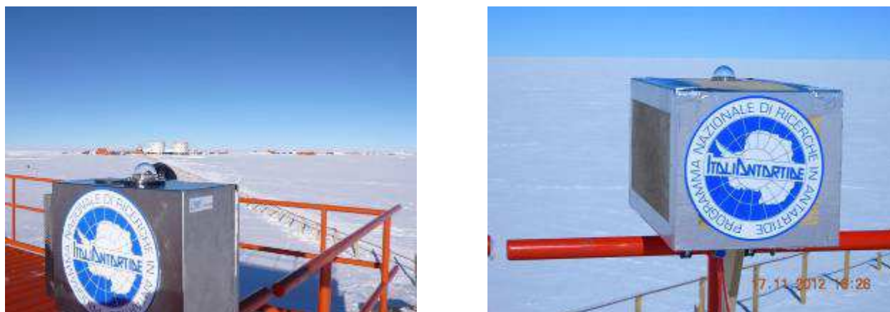
Fig. 1. Filter radiometer (mod. DC-FRAD) located at Dome Concordia, Physics shelter. In the left the instrument without the shield, in the right the instrument with the shield.
