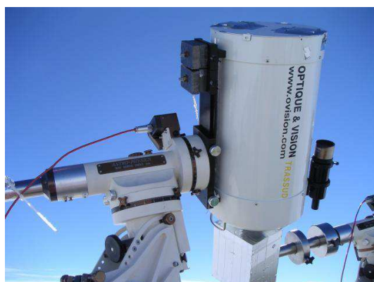
Fig. 1: Left, the DIMM system. Note the 2 hole mask at the telescope top. The box at telescope back contains the camera. Right : typical short-exposure frame of the star Canopus at the focus. The two images move with turbulence. Analysis of their differential motion provides the seeing.
