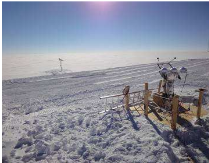
Fig. 1: Status of the BSRN area at the end of the 2011-2012 summer campaign. Tracker and albedo rack.
