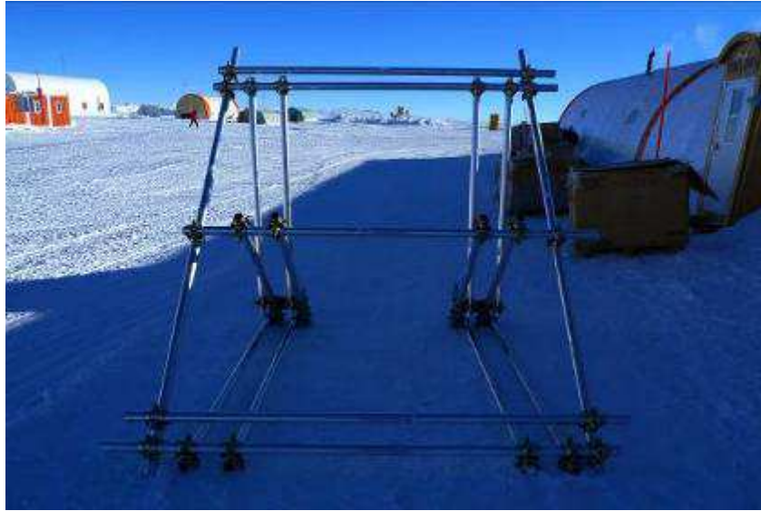
Fig. 3. The metallic structure that joins the radiometer to the American Tower.
