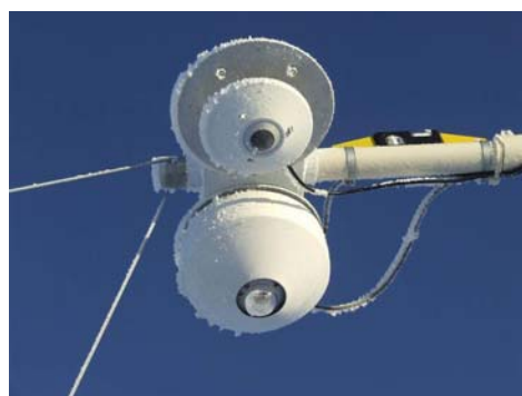
The UV-RAD radiometer developed at ISAC-CNR measuring UV radiation in 7 very narrow channels (<1 nm FWHM)
