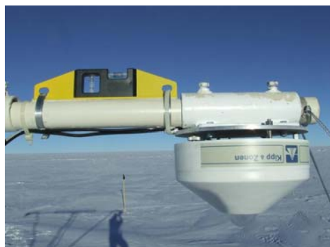
The UV-RAD radiometer developed at ISAC-CNR measuring UV radiation in 7 very narrow channels (<1 nm FWHM)
